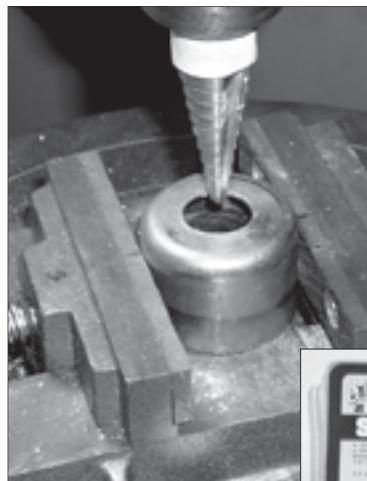
Drill press used for 3/4" hole to accept socket made with step drills from Harbor Freights.
